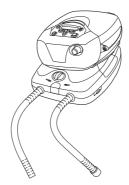
**4** Connect the free end of the medium air tubing to the VPAP Adapt SV. Connect the pressure sensor tube by twisting the Luer lock onto the VPAP Adapt SV (see page 9).
